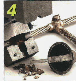
4 Open the mould and remove the expended steel cup – no special disposal required
