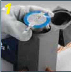
1 Insert CADWELD® PLUS package into mould
