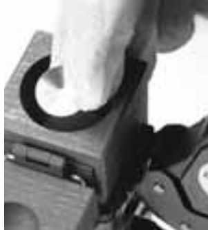
Step 2 Close mould and drop metal disk in place
