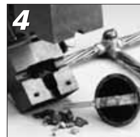
4 Open the mould and remove the expended steel cup – no special disposal required
